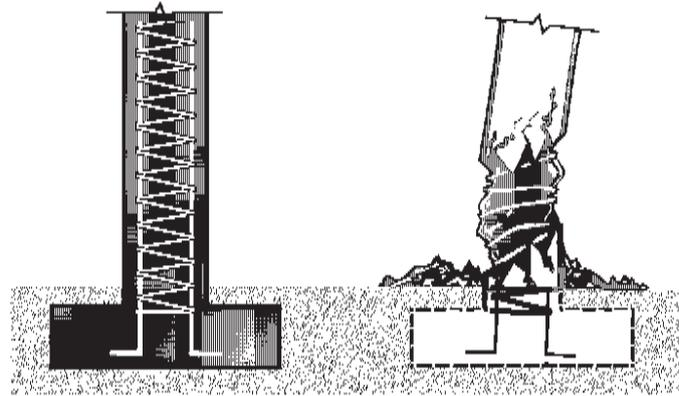
**Figure 21 –Lack of Reinforcing steel.** If the confining reinforcing steel in a column is too widely spaced (a), it will not be able to keep the vertical reinforcing bars and the concrete in place when it is shaken by an earthquake (b).
