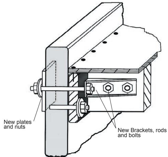
**Figure 14 —Strengthening Wall Anchors.** One of several ways to strengthen the connections between the roof and floor joists and the walls is to install brackets and rods that go through the walls and attach to the joists.
