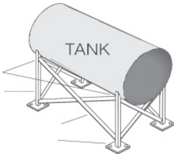
**Figure 49—Bracing tanks.** Tank supports should be cross-braced as well as bolted to the floor.
